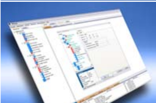
RiZone “Autodiscovery” module – RimatriX5 components are automatically detected in the network.
